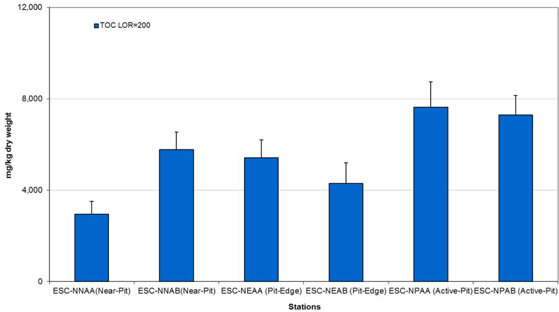
Figure 13: Concentration of Total Organic Carbon (TOC) (mg/kg dry weight; mean +SD) in sediment samples collected from Pit Specific Sediment Chemistry Monitoring for ESC CMP Vd in July 2019.
