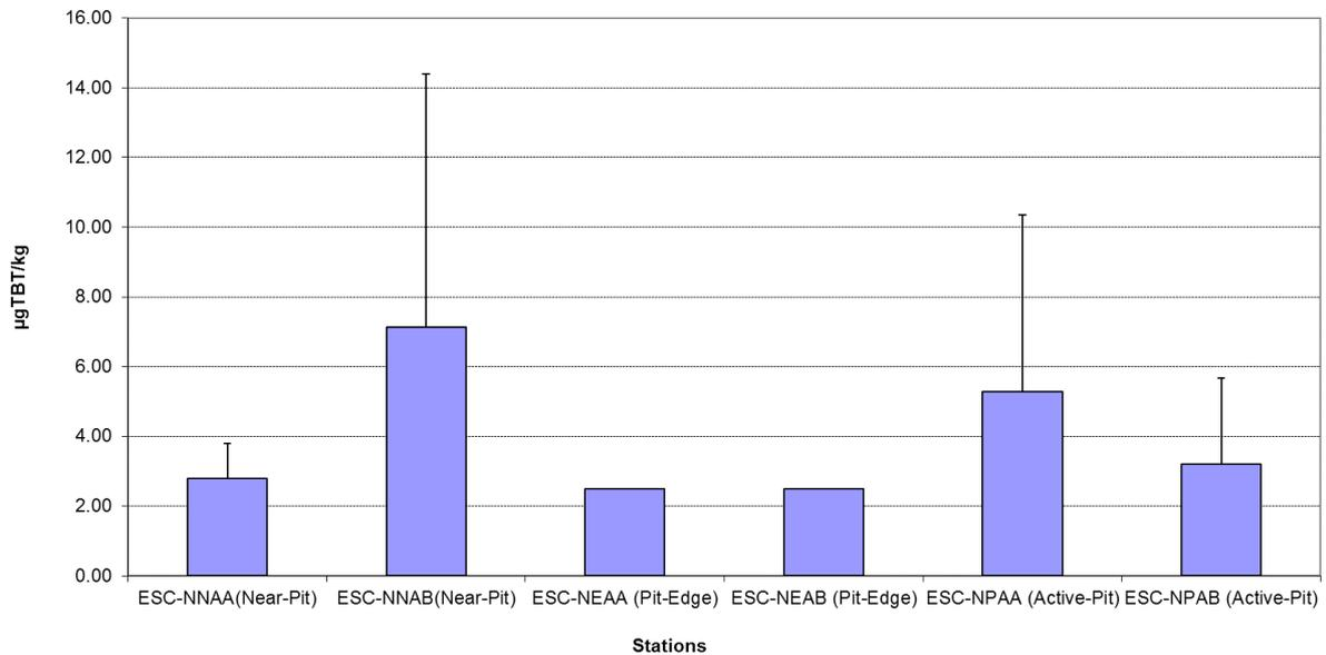
Figure 14: Concentration of Tributyltin (TBT) (µg TBT/kg; mean +SD) in sediment samples collected from Pit Specific Sediment Chemistry Monitoring for ESC CMP Vd in July 2019.
