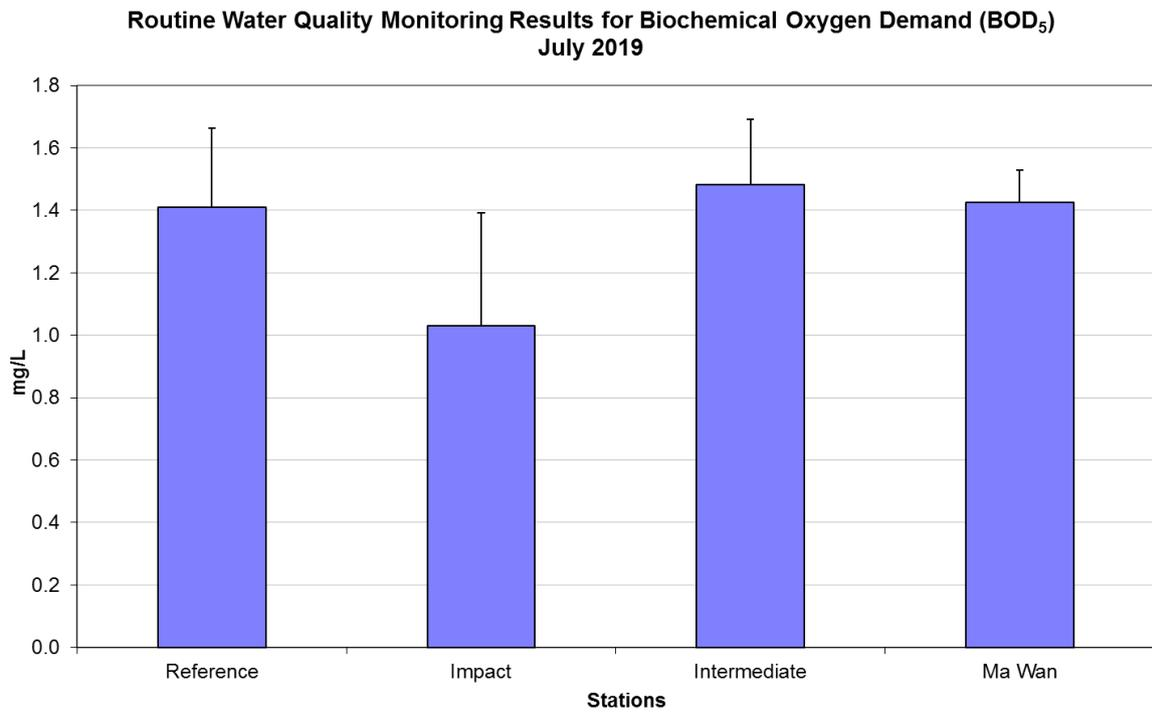
Figure 9: Level of Biochemical Oxygen Demand (BOD<sub>5</sub>) (mg/L; mean + SD) in water samples collected from Routine Water Quality Monitoring for disposal operations at ESC CMP V in July 2019.
