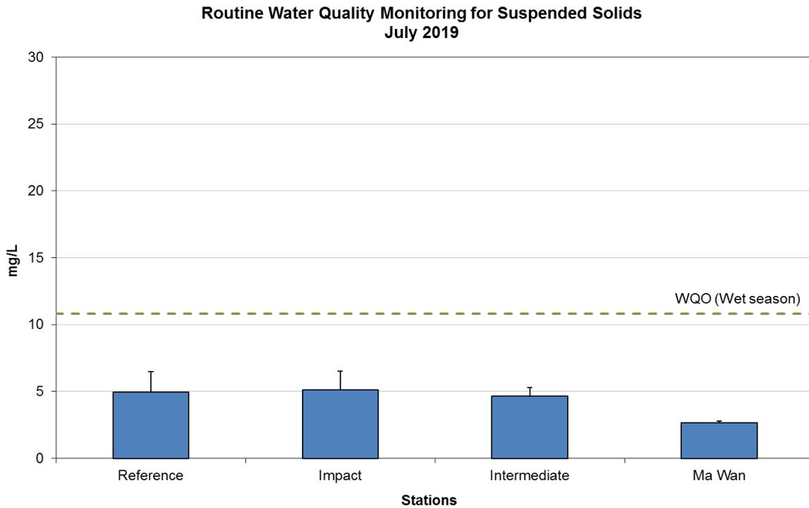
Figure 10: Concentration of Suspended Solids (SS) (mg/L; mean + SD) in water samples collected from Routine Water Quality Monitoring for disposal operations at ESC CMP V in July 2019.
