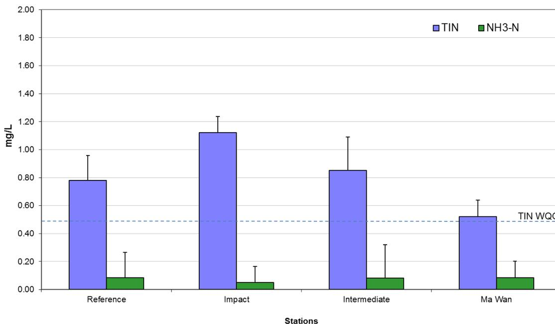
Figure 8: Concentration of Total Inorganic Nitrogen (TIN) and Ammonia Nitrogen ( $\text{NH}_3\text{-N}$ ) ( $\mu\text{g/L}$ ; mean + SD) in water samples collected from Routine Water Quality Monitoring for disposal operations at ESC CMP V in July 2019.
