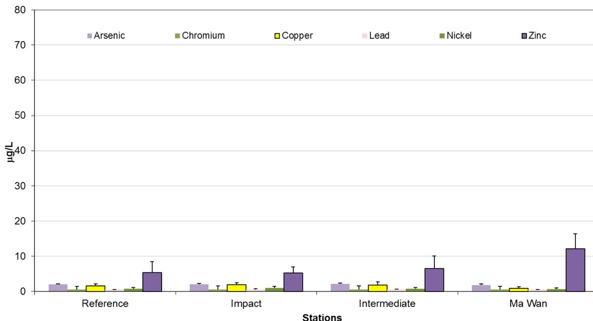
Figure 7: Concentration of Arsenic, Chromium, Nickel, Lead, Copper and Zinc ( $\mu\text{g/L}$ ; mean + SD) in water samples collected from Routine Water Quality Monitoring for disposal operations at ESC CMP V in July 2019.
