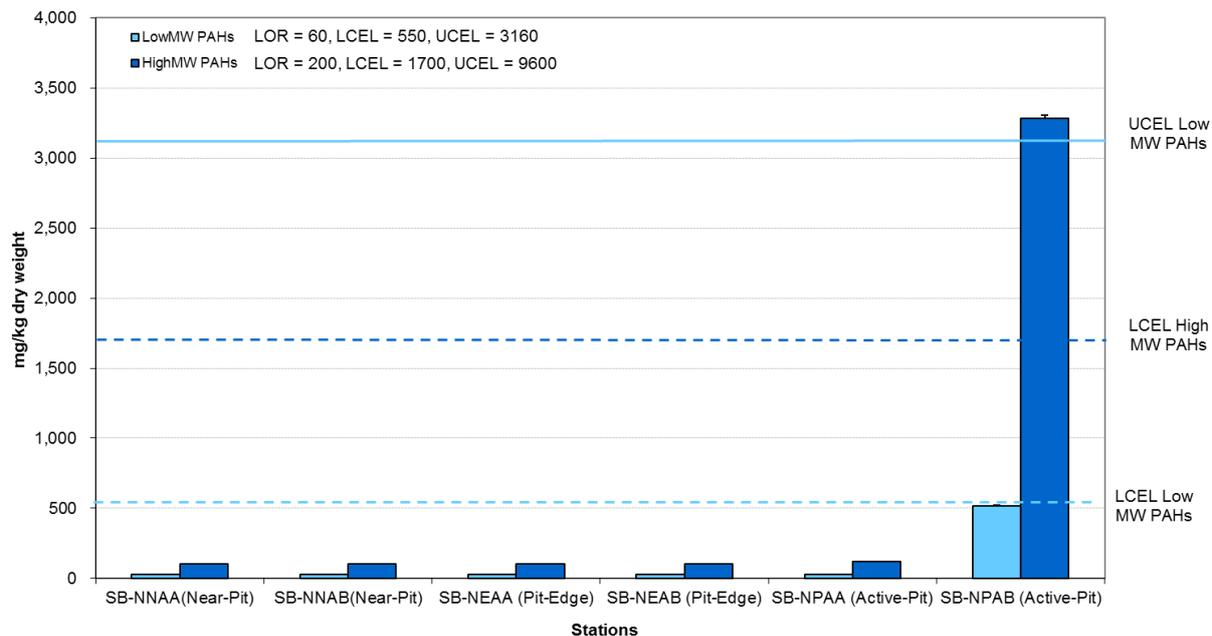
Figure 28: Concentration of Low and High Molecular Weight Polycyclic Aromatics Hydrocarbons (mg/kg dry weight; mean +SD) in sediment samples collected from *Pit Specific Sediment Chemistry Monitoring* for CMP 1 in November 2013.
