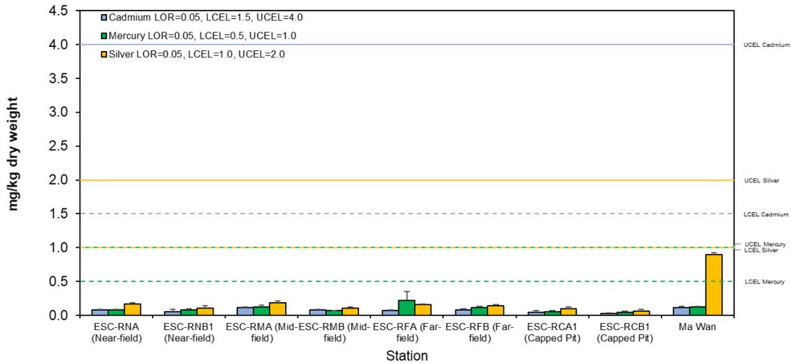
**Figure 17:** Concentration of Metals (Cd, Hg, Ag; mg/kg dry weight; mean + SD) in sediment samples collected from Cumulative Impact Sediment Chemistry Monitoring for ESC CMPs in December 2021
