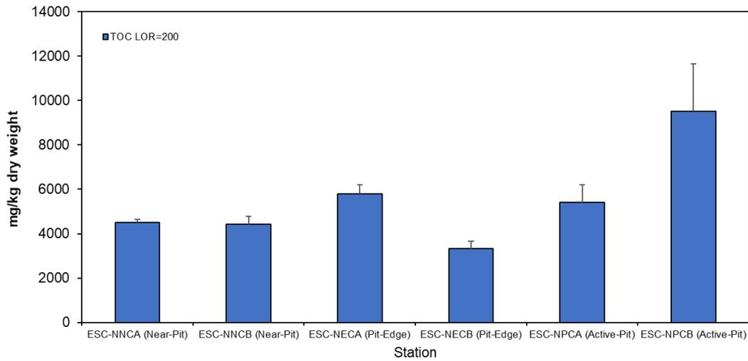
**Figure 13:** Concentration of Total Organic Carbon (TOC) (mg/kg dry weight; mean + SD) in sediment samples collected from Pit Specific Sediment Chemistry Monitoring for ESC CMP Vb in December 2021
