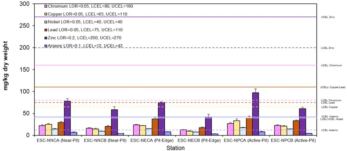
**Figure 11:** Concentration of Metals and Metalloid (Cr, Cu, Ni, Pb, Zn, As; mg/kg dry weight; mean + SD) in sediment samples collected from Pit Specific Sediment Chemistry Monitoring for ESC CMP Vb in December 2021
