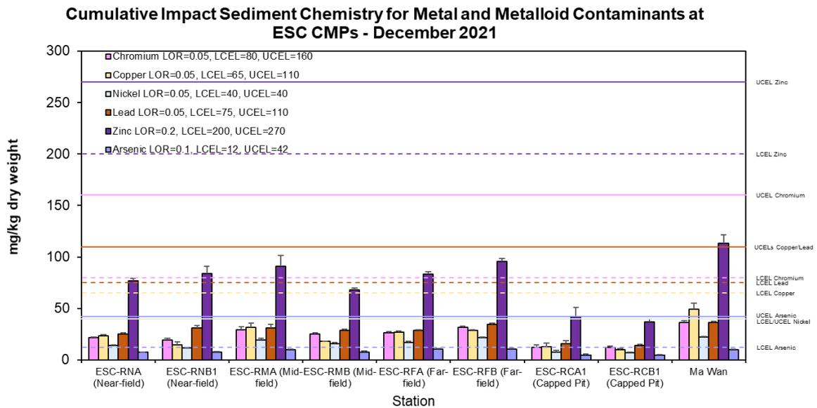
**Figure 16:** Concentration of Metals and Metalloid (Cr, Cu, Ni, Pb, Zn, As; mg/kg dry weight; mean + SD) in sediment samples collected from Cumulative Impact Sediment Chemistry Monitoring for ESC CMPs in December 2021
