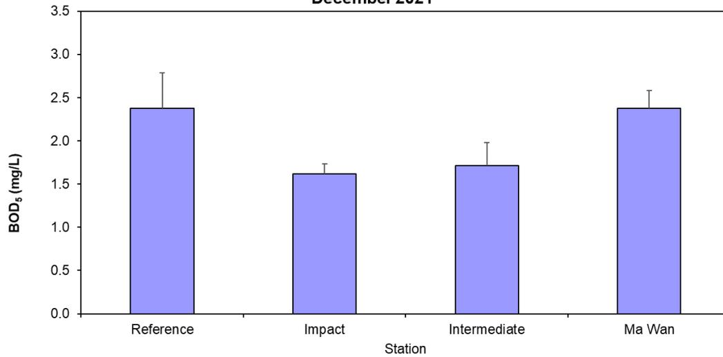
**Figure 9:** Level of Biochemical Oxygen Demand (BOD<sub>5</sub>) (mg/L; mean + SD) in water samples collected from Routine Water Quality Monitoring for disposal operations at ESC CMP V in December 2021
