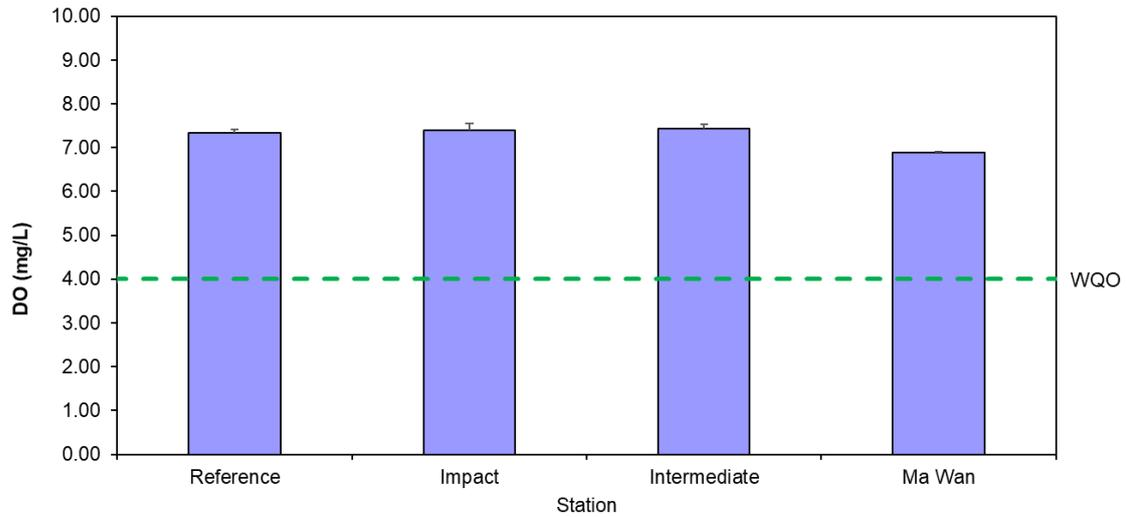
**Figure 3:** Concentration of Dissolved Oxygen (DO) (mg/L; mean + SD)<sup>1</sup> recorded during Routine Water Quality Monitoring for disposal operations at ESC CMP V in December 2021
