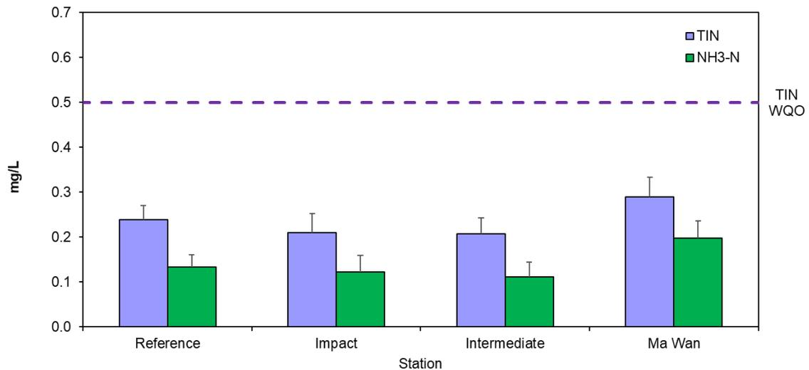
**Figure 8:** Concentration of Total Inorganic Nitrogen (TIN) and Ammonia Nitrogen (NH3-N) (mg/L; mean + SD) in water samples collected from Routine Water Quality Monitoring for disposal operations at ESC CMP V in December 2021
