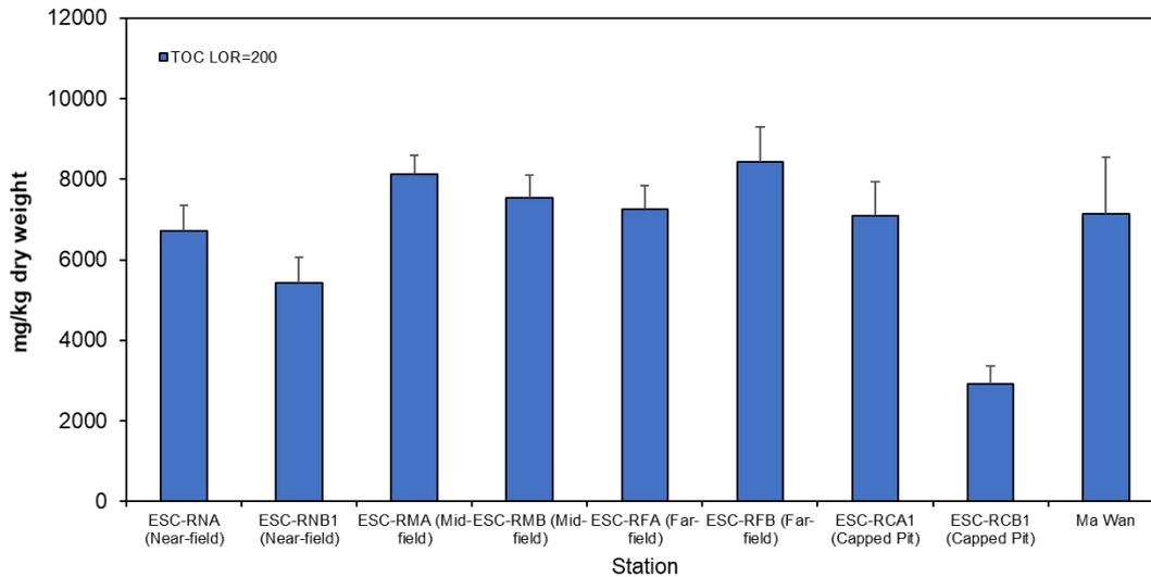
**Figure 18:** Concentration of Total Organic Carbon (TOC) (mg/kg dry weight; mean + SD) in sediment samples collected from Cumulative Impact Sediment Chemistry Monitoring for ESC CMPs in December 2021
