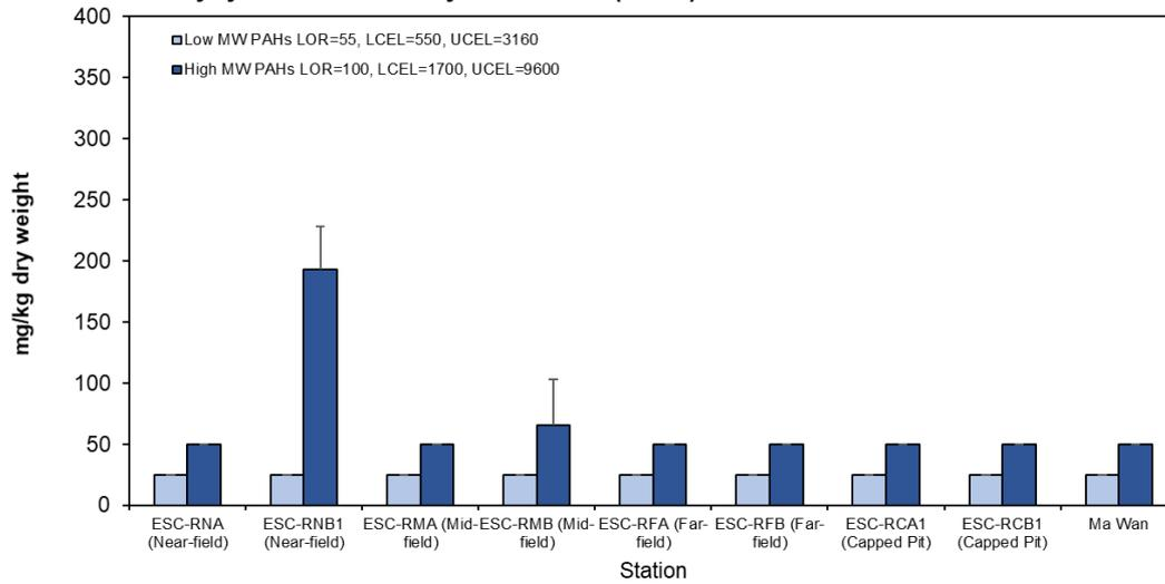
**Figure 19:** Concentration of Low and High Molecular Weight Polycyclic Aromatics (mg/kg dry weight; mean + SD) in sediment samples collected from Cumulative Impact Sediment Chemistry Monitoring for ESC CMPs in December 2021
