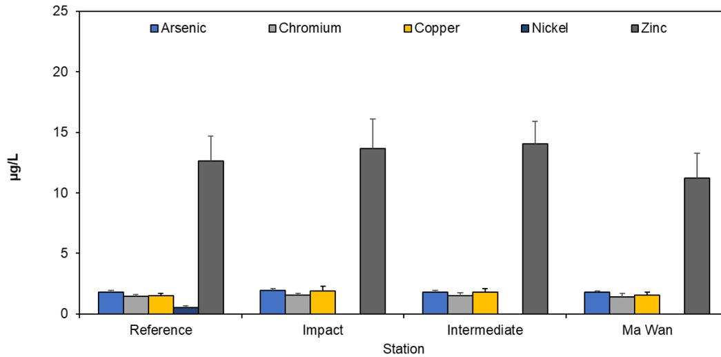
**Figure 7:** Concentration of Arsenic, Chromium, Copper, Nickel, and Zinc (µg/L; mean + SD) in water samples collected from Routine Water Quality Monitoring for disposal operations at ESC CMP V in December 2021
