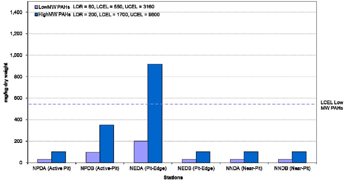
Figure 5: Concentration of Low and High Molecular Weight Polycyclic Aromatics Hydrocarbons (PAHs) ( $\mu\text{g}/\text{kg}$ ; mean +SD) in sediment samples collected from Pit Specific Sediment Chemistry Monitoring for CMP Va in April 2013.
