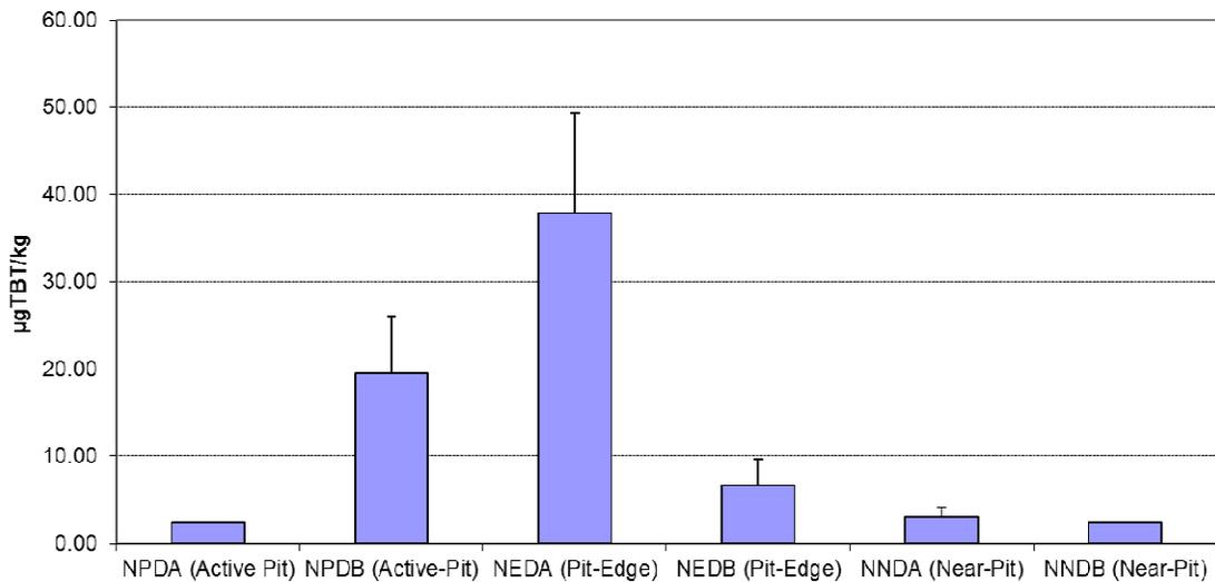
Figure 4: Concentration of Tributyltin (µg TBT/kg; mean +SD) in sediment samples collected from Pit Specific Sediment Chemistry Monitoring of CMP Va in April 2013.
